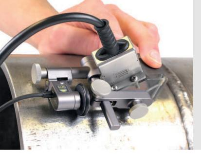
**AXYS** is a universal accessory for single axis inspections, easily set up without any tools.
