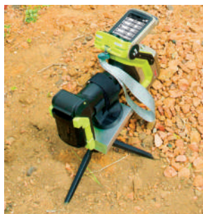
Figure 2. Accessories for the Niton XL5 Plus handheld XRF analyzer: a) Soil guard to protect window bracket b) Tripod for in-situ measurements c) Mini test stand.
