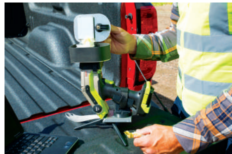
Figure 2. Accessories for the Niton XL5 Plus handheld XRF analyzer: a) Soil guard to protect window bracket b) Tripod for in-situ measurements c) Mini test stand.
