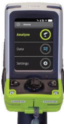
Figure 1. a) Niton XL5 Plus handheld XRF analyzer b) Display of pass/fail result and elemental analysis of soil sample.
