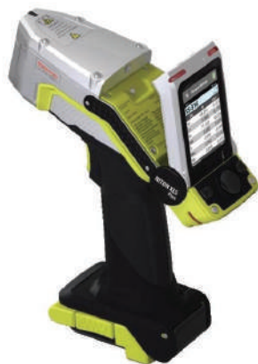
Figure 1. a) Niton XL5 Plus handheld XRF analyzer b) Display of pass/fail result and elemental analysis of soil sample.
