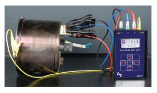
Testing a used EV motor allows for proper evaluation before replacement.
