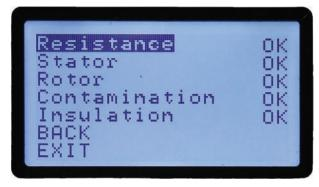
The AT34 EV™ Dynamic Test analyzes the results for you by showing Bad, Warning or OK for Resistance, Stator, Rotor, Contamination, and Insulation.
