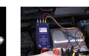
Troubleshoot suspect motors and know immediately if the problem is in the stator, rotor, or connections.
